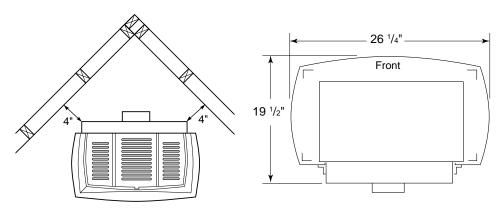
Figure 4 - Clearance for Corner Installation
